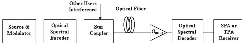
Fig. 2. Schematic of spectral-phase-encoded CDMA using optical amplifier.
