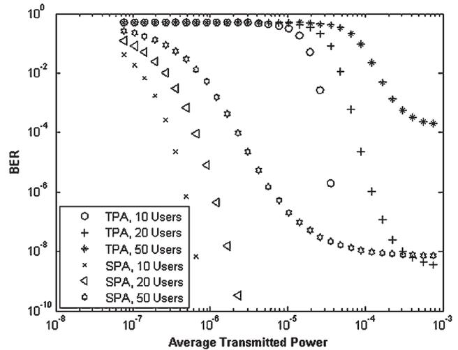
Fig. 8. BER versus average transmitted power for slot-level synchronous transmitters using TPA and SPA receivers with different number of users with a photodetector speed of 2.5 THz.
