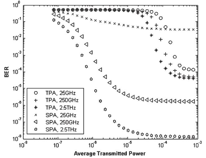
Fig. 3. BER versus average transmitted power for asynchronous transmitters using TPA and SPA receivers with different photodetector speed.
