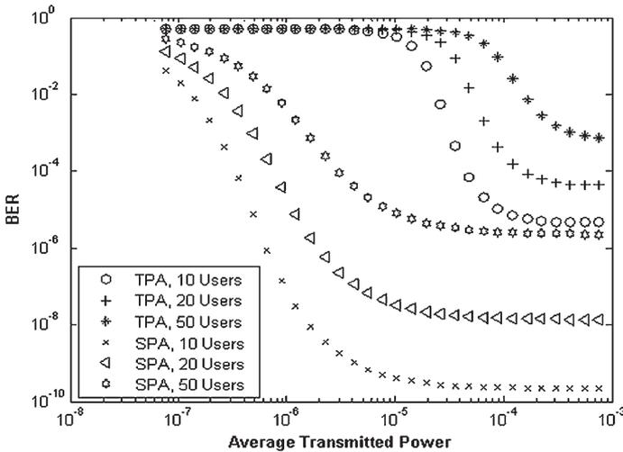
Fig. 6. BER versus average transmitted power for asynchronous transmitters using TPA and SPA receivers with different number of users with a photodetector speed of 2.5 THz.
