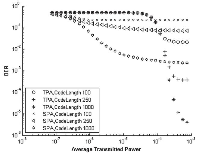
Fig. 11. BER versus average transmitted power for slot-level synchronous transmitters using TPA and SPA receivers with different code lengths with a photodetector speed of 25 GHz.
