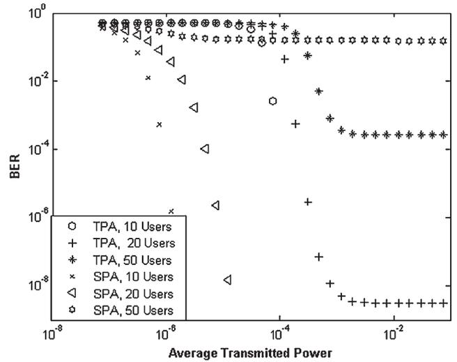
Fig. 7. BER versus average transmitted power for slot-level synchronous transmitters using TPA and SPA receivers with different number of users with a photodetector speed of 25 GHz.
