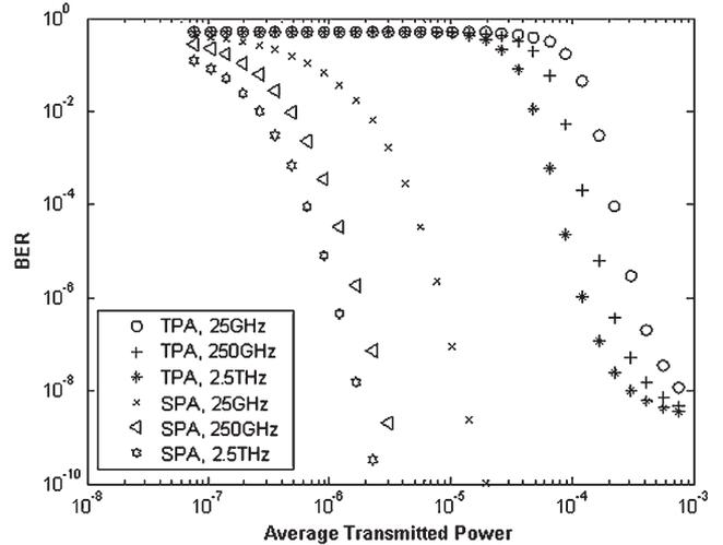
Fig. 4. BER versus average transmitted power for slot-level synchronous transmitters using TPA and SPA receivers with different photodetector speed.
