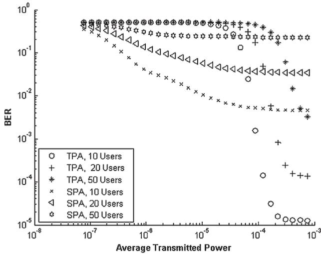
Fig. 5. BER versus average transmitted power for asynchronous transmitters using TPA and SPA receivers with different number of users with a photodetector speed of 25 GHz.
