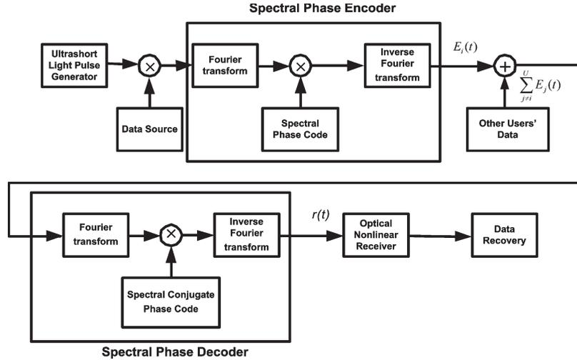
Fig. 1. Typical block diagram of spectral-phase-encoded CDMA.
