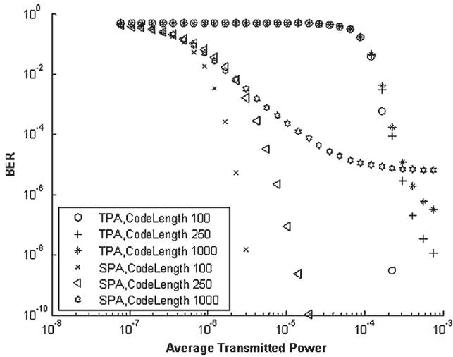
Fig. 9. BER versus average transmitted power for asynchronous transmitters using TPA and SPA receivers with different code lengths with a photodetector speed of 25 GHz.
