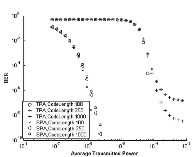
Fig. 12. BER versus average transmitted power for slot-level synchronous transmitters using TPA and SPA receivers with different code lengths with a photodetector speed of 2.5 THz.
