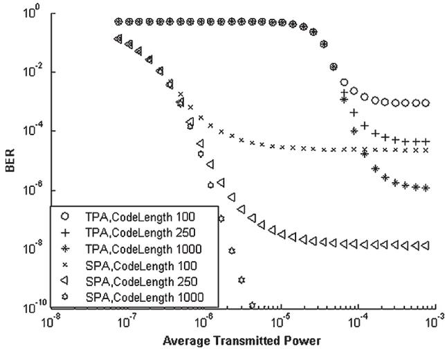
Fig. 10. BER versus average transmitted power for asynchronous transmitters using TPA and SPA receivers with different code lengths with a photodetector speed of 2.5 THz.
