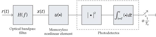
Fig. 1. The general form of the optical nonlinear receiver.
