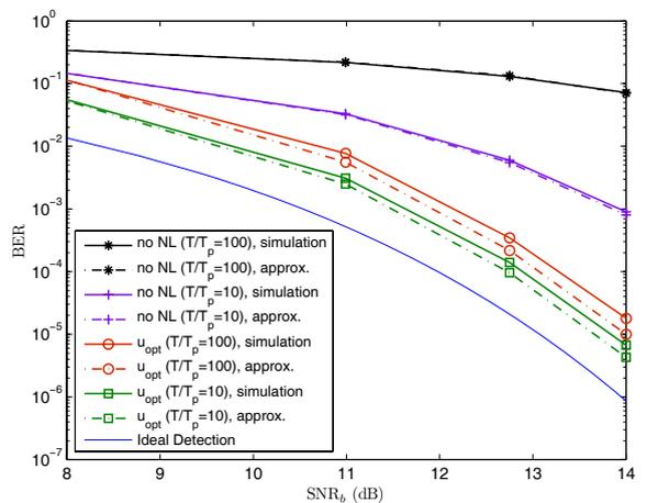
Fig. 4. Performance of the optimum detector, detector with no nonlinearity (NL), and ideal detector.
