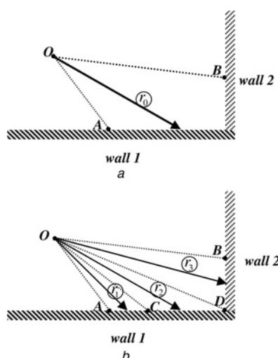
**Figure 1** Space sampling error and its solution
