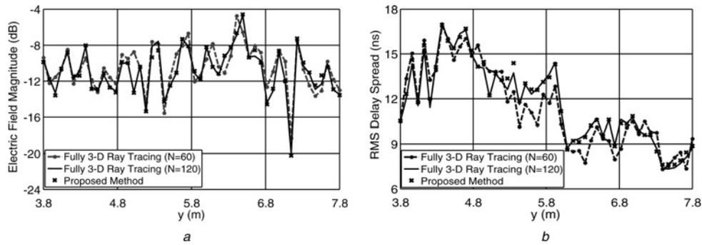
**Figure 8** Radio channel parameters computed by our proposed method and fully 3-D ray tracing with  $N = 60$  compared to the reference solution (fully 3-D ray tracing with  $N = 120$ ) for LOS case
