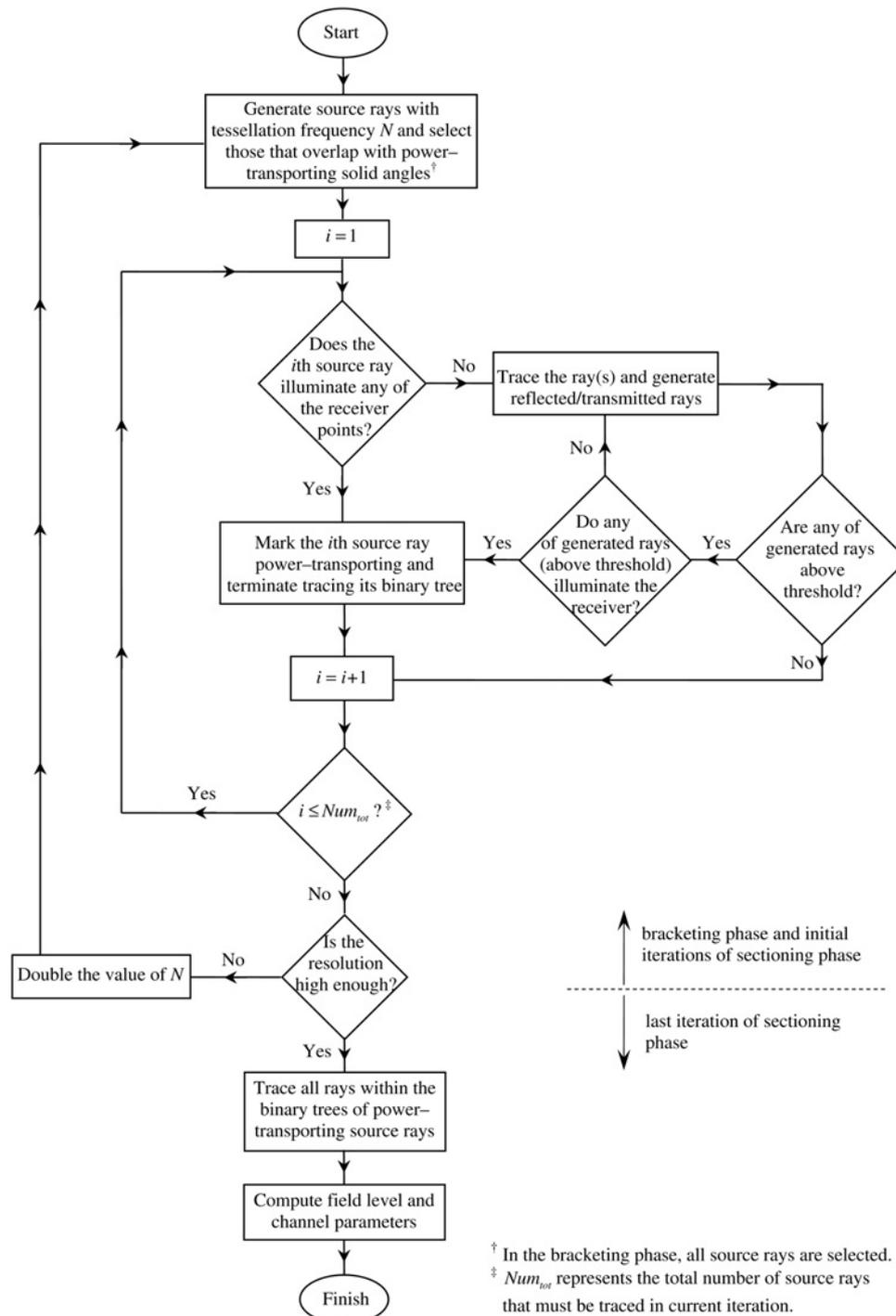
Figure 3 Flowchart of proposed acceleration technique
