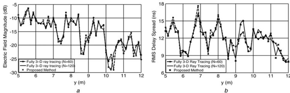
**Figure 9** Radio channel parameters computed by our proposed method and fully 3-D ray tracing with  $N = 60$  compared to the reference solution (fully 3-D ray tracing with  $N = 120$ ) for NLOS case
