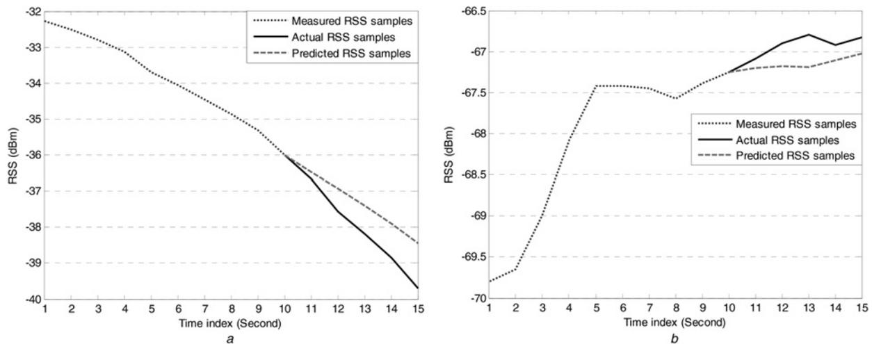
**Fig. 4** Predicted RSS samples based on previous RSS samples using the RLS-based predictor,  $N_{obs} = 10$ ,  $N_{pr} = 5$ ,  $F_l = 5$
