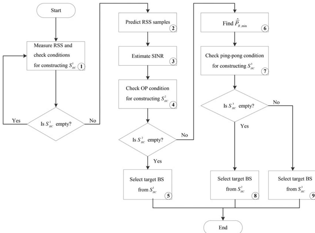
Fig. 3 Flowchart of the proposed algorithm for selecting the target BS
