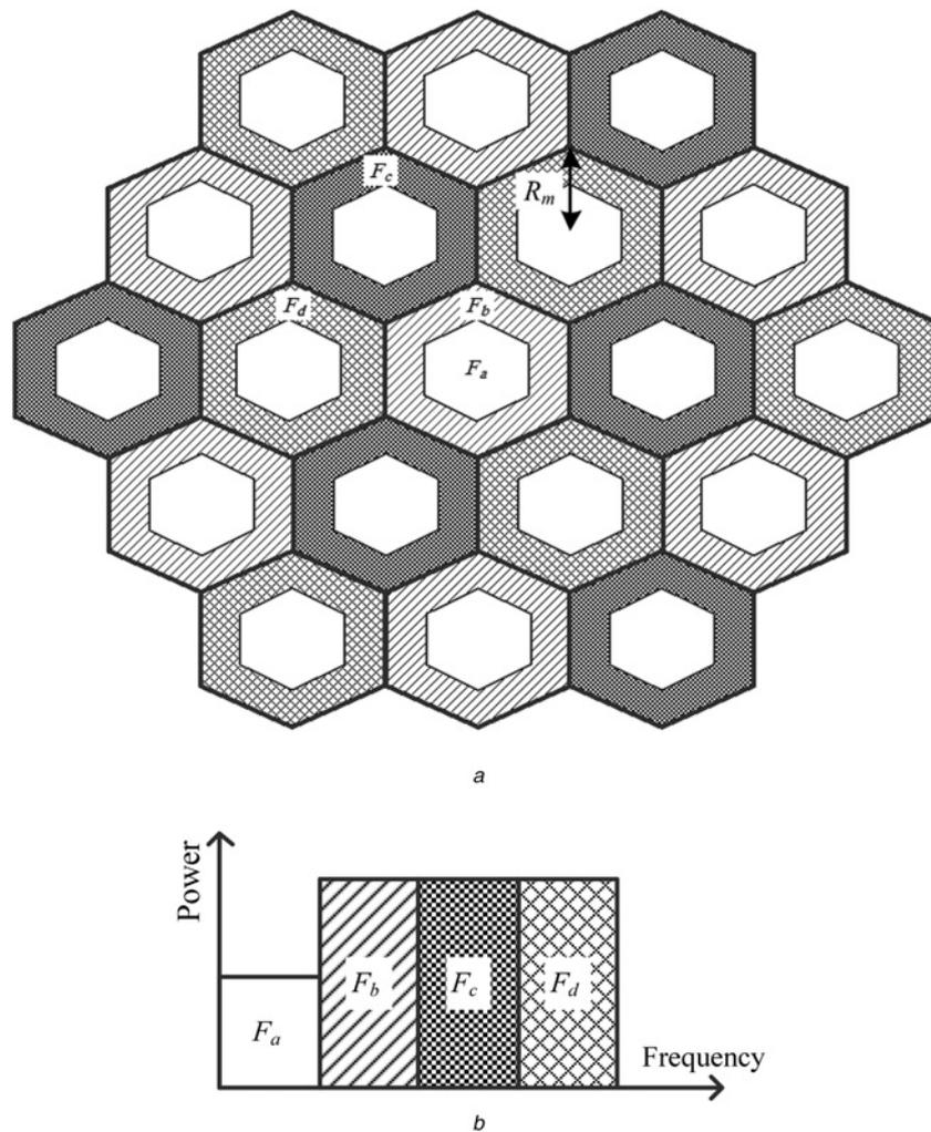
**Fig. 1** Macrocell network layout and frequency partitioning used in this study
