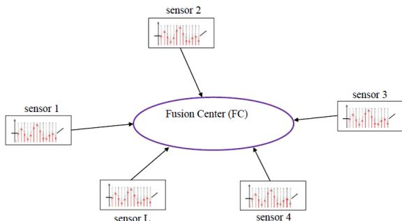
Figure 2: The star topology for centralized recovery.
