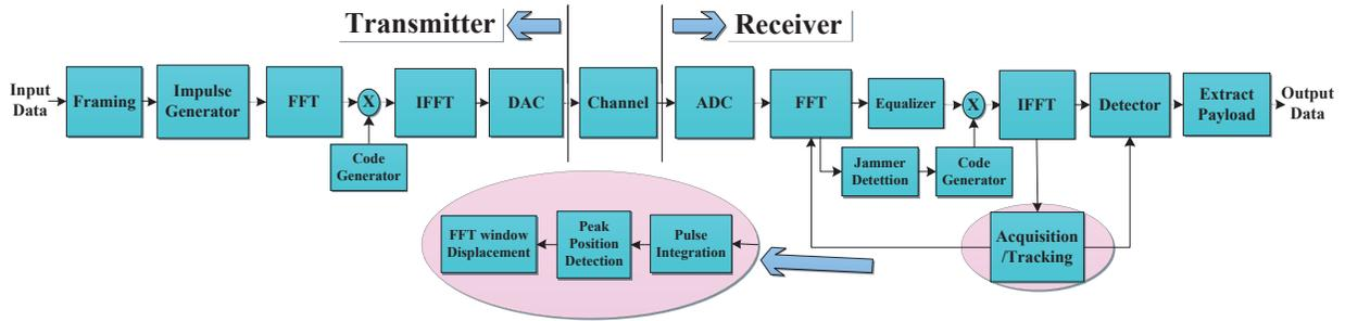
Fig. 1. Block diagram of the implemented SE/ST-CDMA system.
