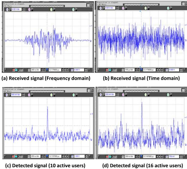
Fig. 3. Signal representations showing the multi user performance of the implemented SE/ST-CDMA system.
