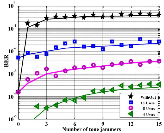
Fig. 6. BER versus the number of jammers for three different number of users, the performance of eight users scenario without jammer cancellation is also shown. (solid lines: simulation, dots: experimental).
