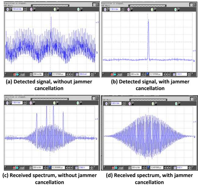
Fig. 4. Signal representations showing the jammer cancellation performance in the implemented SE/ST-CDMA system.
