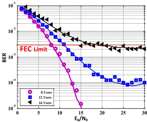
Fig. 5. BER performance versus  $E_b/N_0$  with different number of users (solid lines: simulation, dots: experimental).
