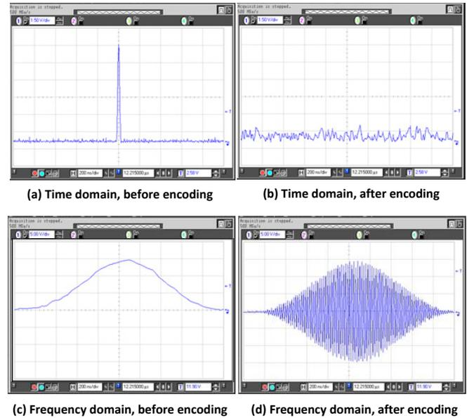
Fig. 2. Transmitted signal's time and frequency domain representation before and after the spectral encoder at the transmitter.
