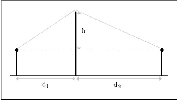
Figure 1. Diffraction Geometry
