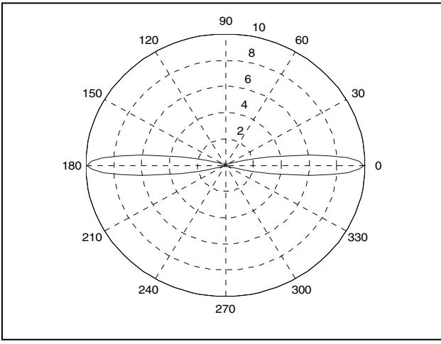
Figure 3. Pattern of directive transmitting antenna
