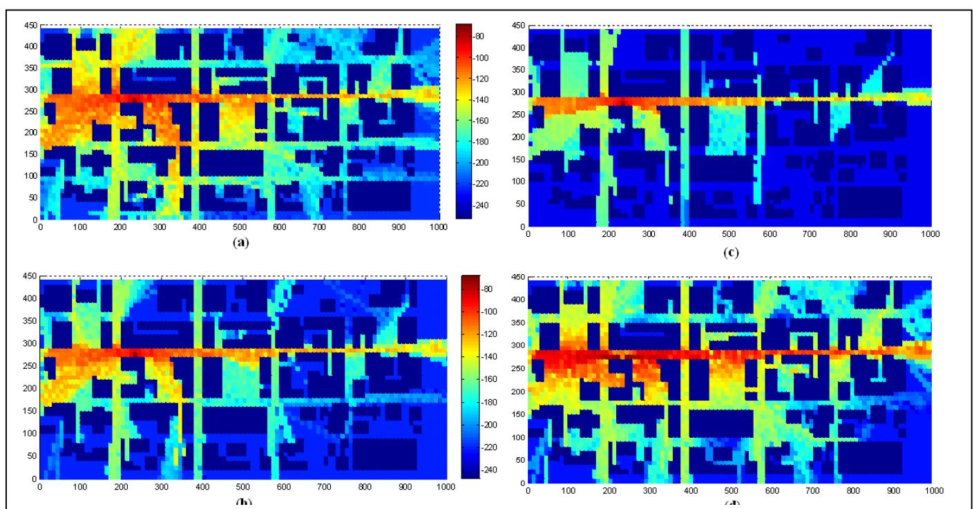
Figure 2. Received power on a bird's eye view of the city in the cases of (a) smooth, (b) rough and (c) very rough wall surfaces with an omni-directional transmitter, and (d) with smooth surfaces and a directive transmitting antenna
